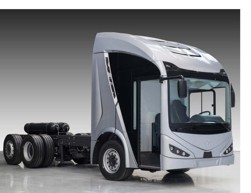
This led to the birth of the Irizar ie truck, a truck designed for different industrial uses in cities with a focus on electromobility. It will initially be used for collecting municipal waste.
