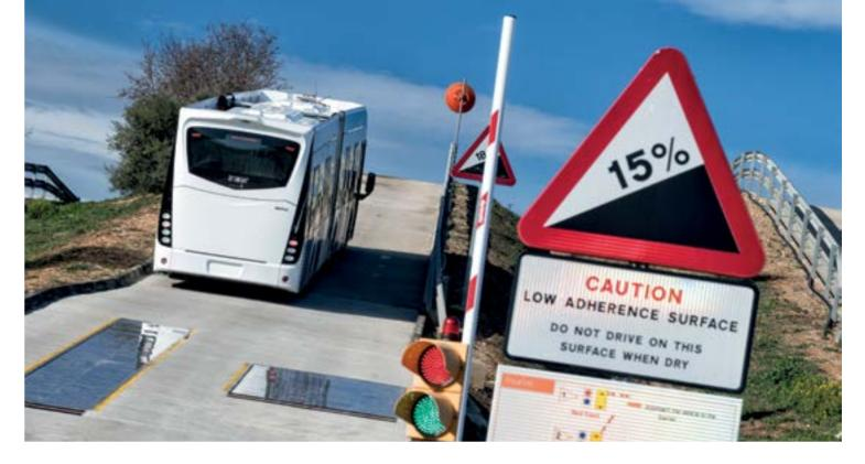
The undulations of the track (symmetrical and asymmetrical on the left and right wheels) test the suspension systems and help in assessing the level of comfort inside the vehicle. Cobblestones, for example, cause a high frequency of large vertical forces that affect the vehicle's suspension systems and structure.
