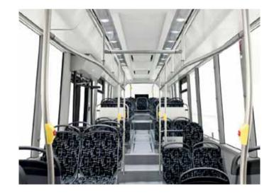
Equipped with an integrated access ramp in the central door, our coach has an area for people with reduced mobility and baby carriages. Its interior design, made using anti-vandalism materials, facilitates cleaning and maintenance. The front is modular and removable, which facilitates replacing components that have a greater risk of damage from accidents.
